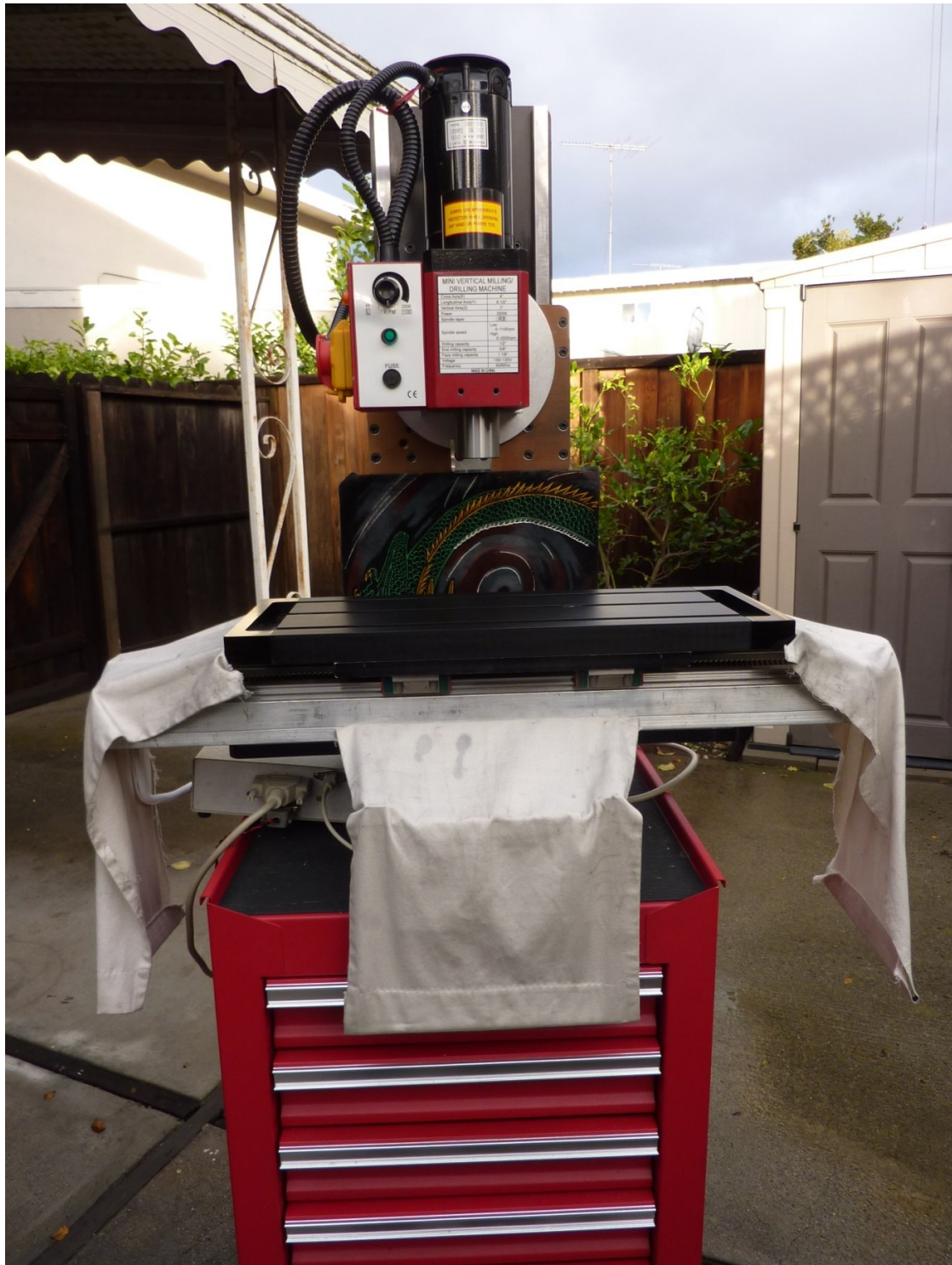
Cloth covers protect lead screw and rails from milling chips.
